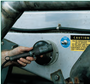
One Connection for Overfill Prevention and Grounding
